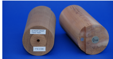
Cedar Insert with Solid Tumour (drilled) Chamber Dosimetry in a Tumour within Lung Density Material
