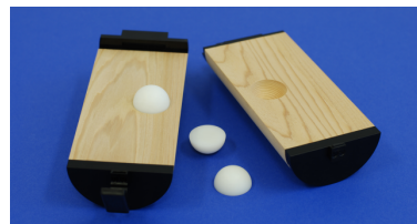
Cedar Ion Chamber Holder Insert (drilled) Chamber Dosimetry within Lung Density Material
